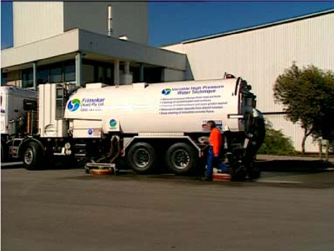
Figure 8 - A Frimokar Australia High Pressure Jet and Suction Cleaning Vehicle in Action
